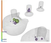
nanoCT® of TSVs in an electronic package. The voids in the copper filling are clearly visible.
