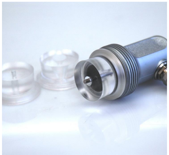
Figure 2: The DYA 5PA32 with modular delay line
