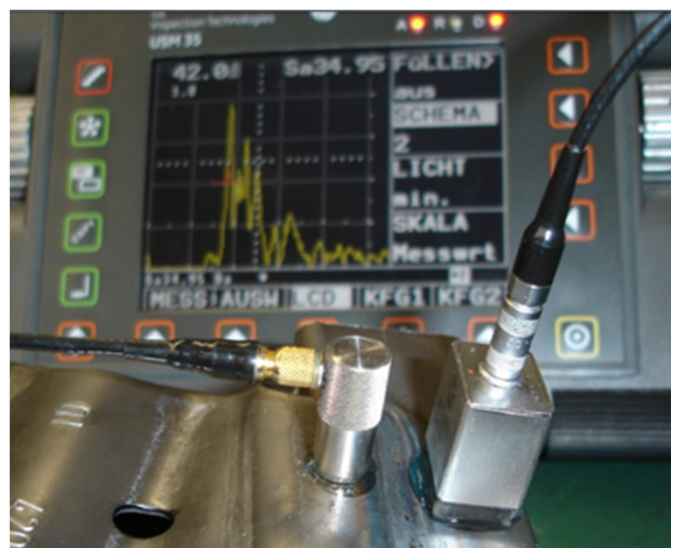
Figure 2: Inspection with A-Scan result
