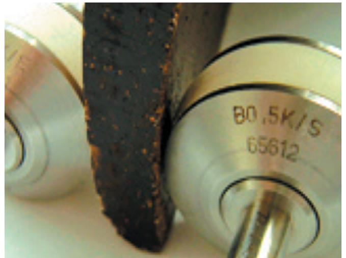
Figure 1: Inspection with roller probes
