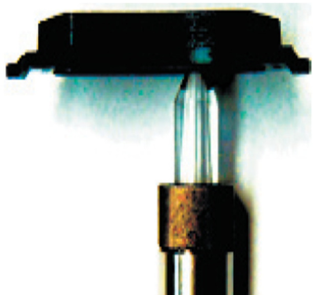
Figure 2: Inspection with squirter probes
