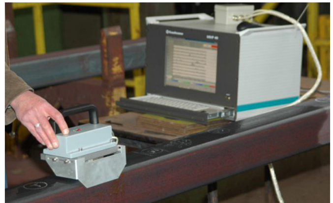
Figure 1: Scanner unit for manual billet testing
