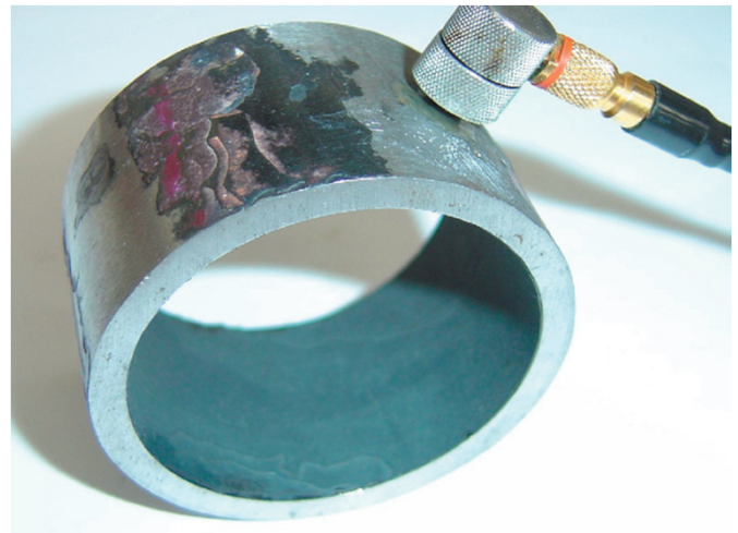
Figure 1: Inspection of a boiler tube
