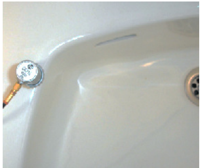
Figure 1: Thickness measurement on a wash basin
