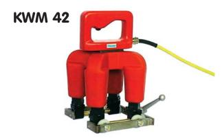
The **cross yoke KWM 42** consists of two AC yokes dis-placed by 90° so that both longitudinal and transverse cracks can be detected in one single operation. Two castors on each magnetic pole maintain a constant air gap and enable the yoke to be moved easily over the test surface.The KWM 42 is powered by a 3-phase supply through a separate transformer.
