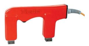
The AC hand yoke **TWM 42 A/N** operates at 42 V supplied from a separate transformer which is connected to a 230 V AC supply. This satisfies the VDE safety regulations so that the TWM 42 A/N can be used for testing invessels, tubes and closed containers.
