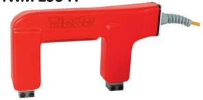
The **TWM 230 A** hand yoke is of similar construction to the TWM-N type, however, the switch on this model can be exchanged when it becomes worn, or faulty. We have also introduced a special switching circuit so that the yoke is switched on when the AC current is passing through zero, thereby greatly extending the life of the switch and the yoke.
