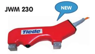
The **hand magnet JWM 230** is small in size, light in weight, and therefore handy to use. Its magnetization output is adequate to satisfy the majority of test requirments. Articulated pole pieces with twinknuckle adjustments may be mounted on the yoke to extend the range of test applications and to ensure the optimum development of the magnetic field within the test piece.
